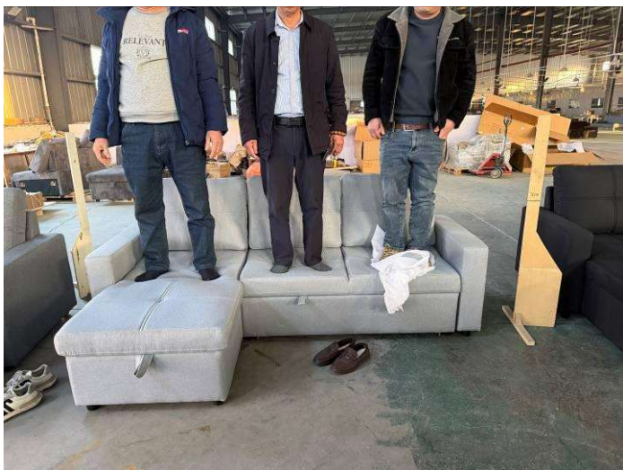
Product load bearing test ( About 240kg )
