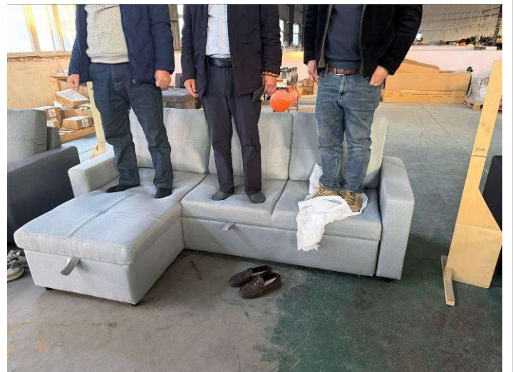
Product load bearing test ( About 240kg )
